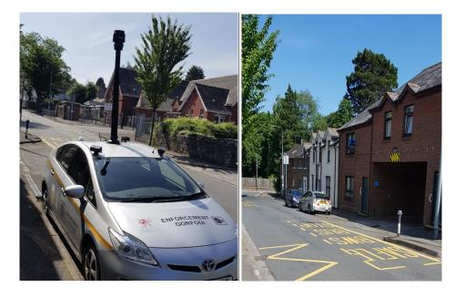
Cars are fitted with rooftop CCTV and Automatic Number Plate Recognition technology and operate 7 days a week between 7am and 10pm. Specific emphasis is placed on illegal parking around schools in order to improve road safety and change driving habits in Cardiff.
